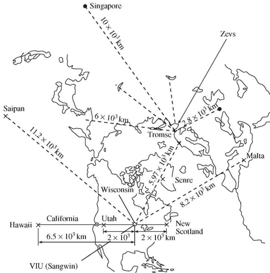
Fig. 1. Arrangement of the Sangwin and “Zevs” ELF antennas and the location of detection sites.
