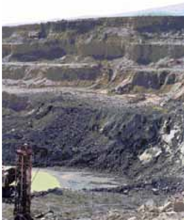
Fig. 19. The Sopcheozero chromite deposit mine, upper banks opened moraine (light colour), lower banks opened chromitite (black).
