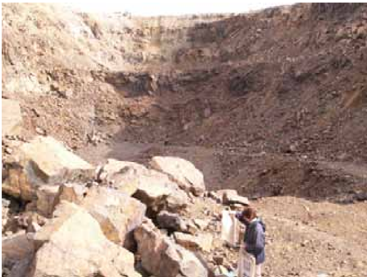
Fig. 25. Mine of the Nud-II deposit. The walls of the mine and dumps contain numerous debris of sulphide nests and disseminated ores.
